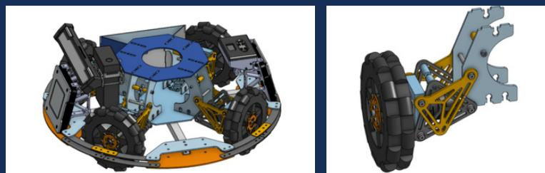
As Infantry and Sentry share very similar chassis designs, they have been designed and prototyped in parallel. This new chassis design focuses on rigidity and ease of manufacturing. It also features easier to access electronics bays, a sturdier aluminum bumper ring, and armor panels that can be easily staggered to throw off enemy robots.
